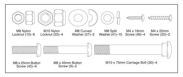
Identify the Front Stabilizer (2). See the inset drawing. Attach a Wheel (14) to one end of the Front Stabilizer with an M8 Nylon Locknut (10). Make sure that the Wheel is oriented as shown and that it turns freely. Next, align the four plastic posts on a Wheel Cover (23) with the plastic posts on the Wheel, and press the Wheel Cover onto the Wheel. Assemble the other Wheel (not shown) in the same way.
